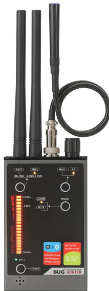
The VS80's front panel: dual antennas, magnetic probe, threshold knob, and full control layout
