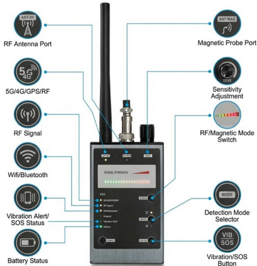
Every button, port, and indicator on the V90 front panel and top edge
